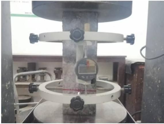
(c) 棱柱体弹性模量试验
