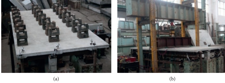
FIGURE 5: Pictures of the static tests: (a) weight loading test; (b) hydraulic loading test.
