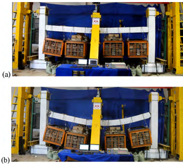
Fig. 6. Failure mode of RC specimen at the end of the 6th load step: (a) damage condition at the end of the test; (b) collapse condition after 20 min of the test.
