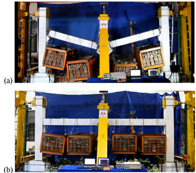
Fig. 5. Failure mode of specimens at the end of the 4th load step: (a) PC specimen; (b) RC specimen.
