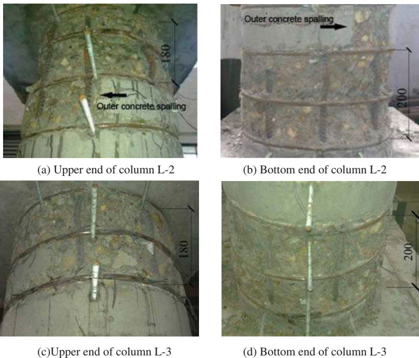
FIGURE 20 Demonstration of the length of plastic hinge.
