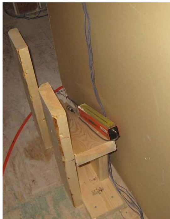
Fig. 3. Diagonal deformation measurements using stringpot
