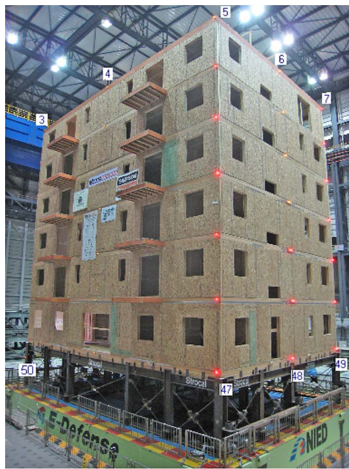
Fig. 4. Optical tracking system to record absolute displacements during testing
