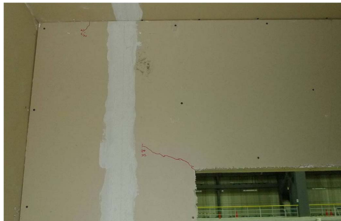
Fig. 8. Minor crack on Wall E4, Story 2 (over window opening) after Level 1 shaking
