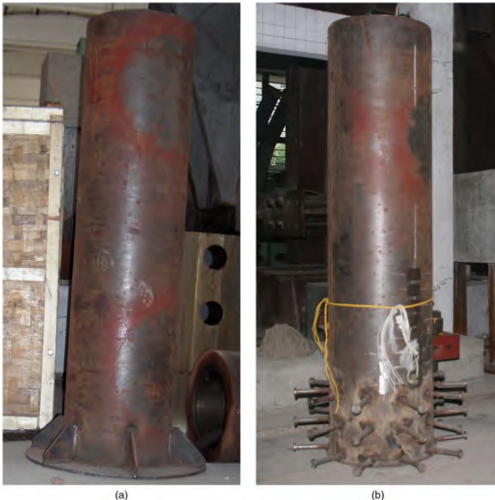
Fig. 1. Steel tube base details: (a) stiffened end plate; (b) studs (images by the authors)
