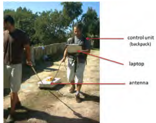
Fig. 5. Main components of a GPR system: control unit, laptop and antenna.
