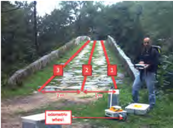
Fig. 6. The GPR survey consisted of three parallel profiles 1 m apart using 500 and 250 MHz shielded antennas.
