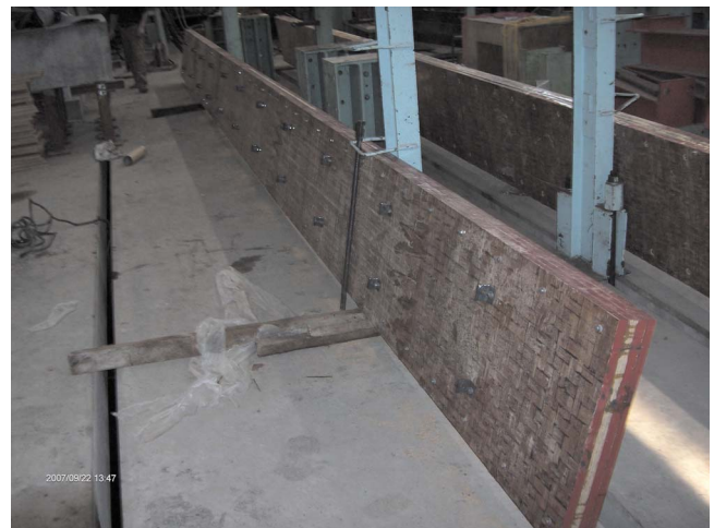
Fig. 1. Laminated bamboo girder
