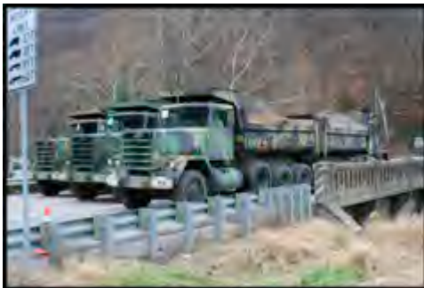
Fig. 4. Picture of six trucks during the load test
