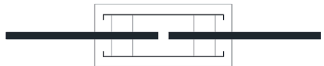
Fig. 9. Double-sided pull-out test specimen.
